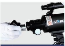
7. Install the Zenith mirror into the end of the main scope tube.
