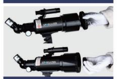
11. Remember to remove the lens dust protectors before observing.
