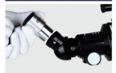
9. Insert the eyepiece (25mm eyepiece is recommended first). Please note, prior to inserting the eyepiece you can insert the Barlow Lens into the Zenith Mirror, this will improve your magnification 3x
