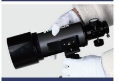
3. Align the screw hole, under the main scope, to the tripod screw.
